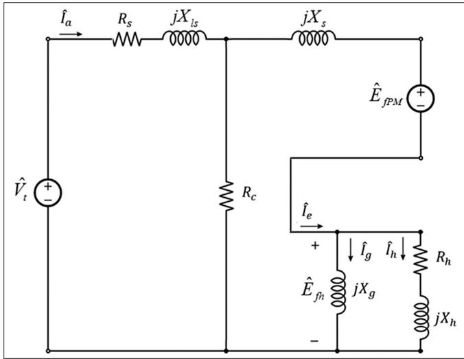
**Fig. 3.** Equivalent circuit of the disc-type double-sided PMHS motor.
