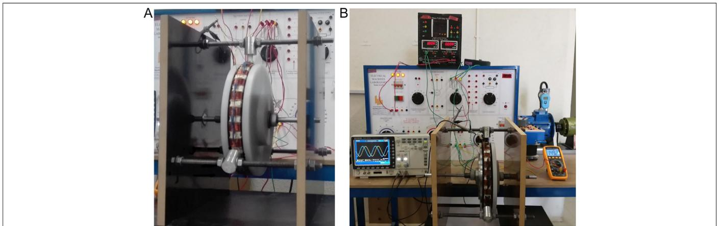
**Fig. 4.** (a) Built hysteresis motor. (b) Test stand for the PMHS motor.
