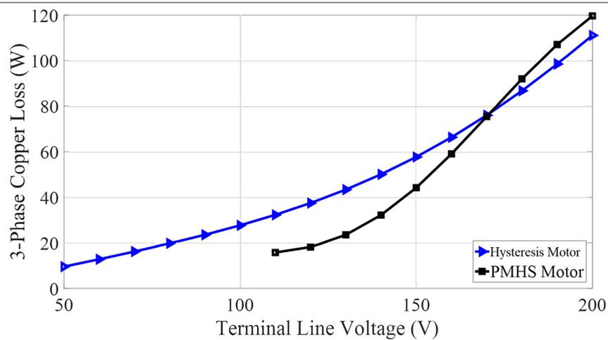
**Fig. 8.** Variations of copper loss versus input line voltage for hysteresis motor and PMHS motor.
