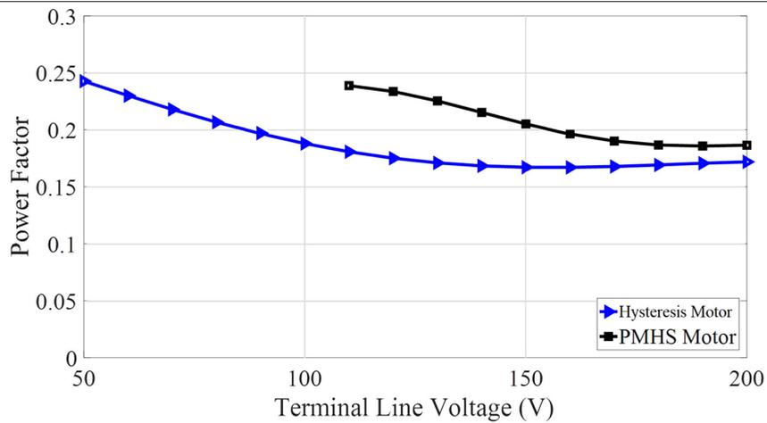
**Fig. 6.** Variations of power factor versus input line voltage for hysteresis motor and PMHS motor.
