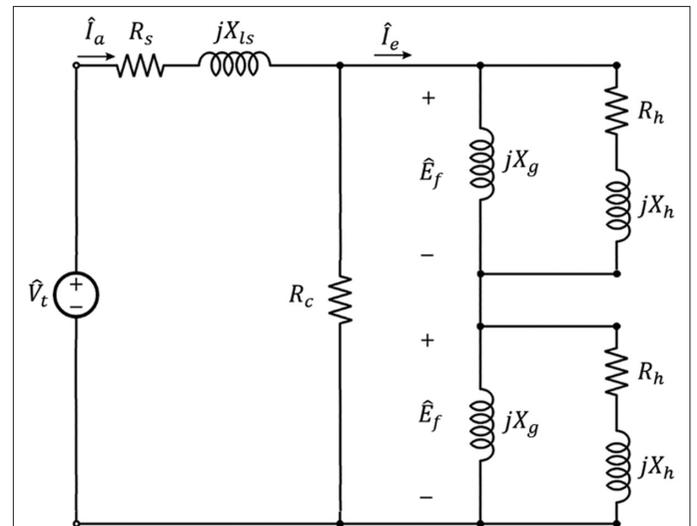
**Fig. 2.** Equivalent circuits of double-sided disc-type hysteresis motor.
