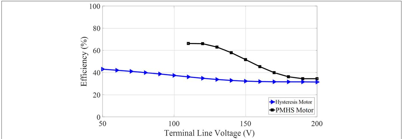
**Fig. 9.** Variations of motor efficiency versus input line voltage for hysteresis motor and PMHS motor.
