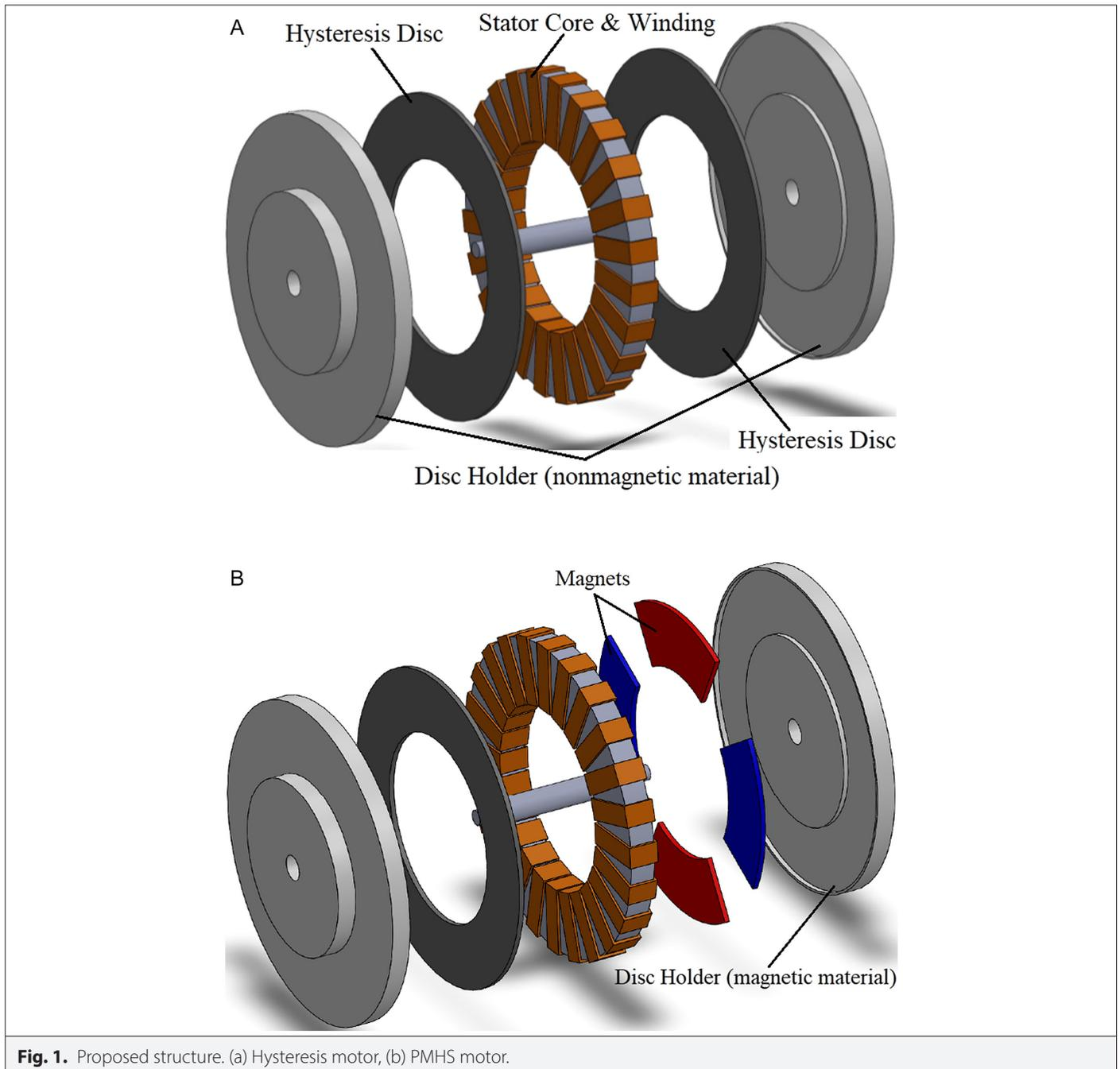
**Fig. 1.** Proposed structure. (a) Hysteresis motor, (b) PMHS motor.
