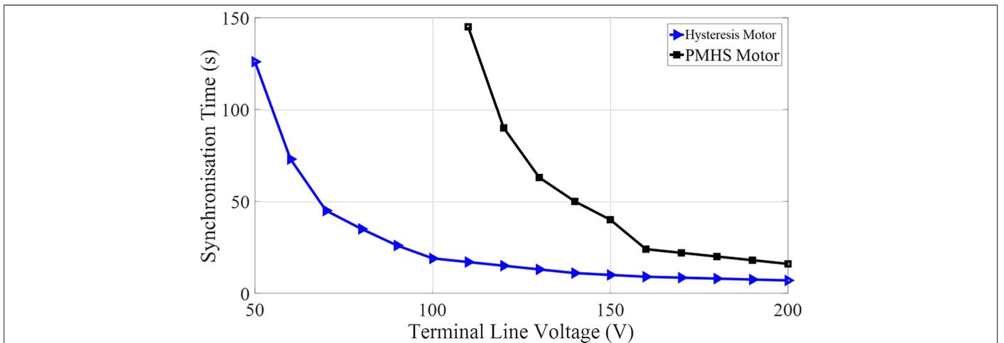
**Fig. 10.** The synchronisation time variations curve with respect to the input line voltage for hysteresis motor and PMHS motor.
