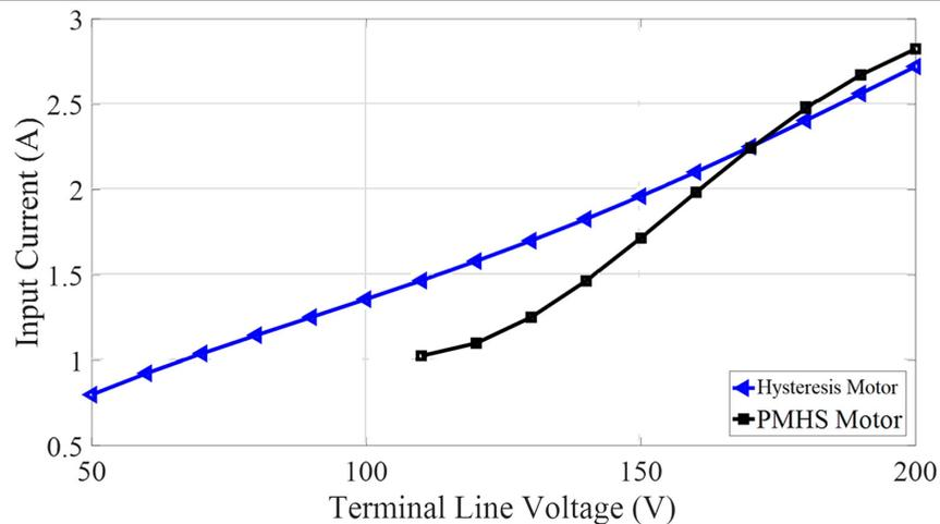
**Fig. 5.** Variations of input current versus input line voltage for hysteresis motor and PMHS motor.
