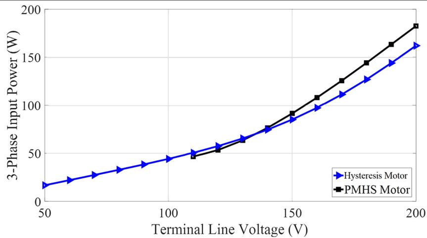
**Fig. 7.** Variations of input power versus input line voltage for hysteresis motor and PMHS motor.
