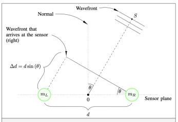
Fig. 1. Geometry of a simple acoustic direction finding system.
